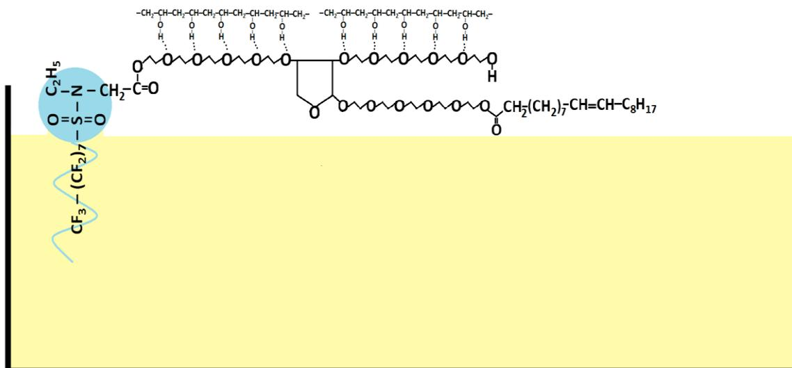
**Fig. 2.** Scheme of the coating formed by the interaction of 2-(N-ethylperfluorooctane sulfamide) acetic acid, sorbitan monooleate, polyethylene glycol and polyvinyl alcohol.
