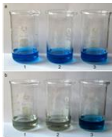
Figure 6. MB solutions ( C = 3 \cdot 10^{-5} mol/l) before (a) and after 20 min treatment with Fenton system ( \text{FeSO}_4 ( C = 3 \cdot 10^{-4} mol/l) + \text{H}_2\text{O}_2 ( C = 4.4 \cdot 10^{-3} mol/l) (b): 1 – control solution, 2 – solution containing guanidine hydrochloride ( C = 3 \cdot 10^{-4} mol/l), 3 – solution containing PHMG-Cl ( C = 3 \cdot 10^{-4} mol/l) ( t = 20^\circ\text{C} )
