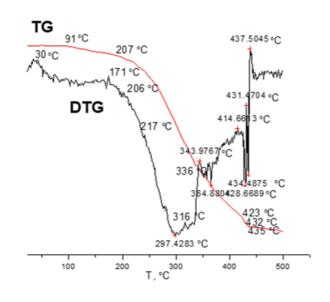
Fig. 2. DTA, TG, and DTG curves of PS-derived FAA.
