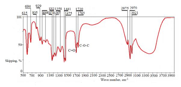
**Fig.5.** IR spectrum of a mixture of 2- (N-ethylperfluorooctansulfamide) acetic acid and polyethylene glycol sorbitan monooleate.
