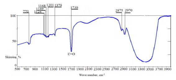
Fig.3. IR spectrum of 2-(N-ethylperfluorooctansulfamide) acetate.
