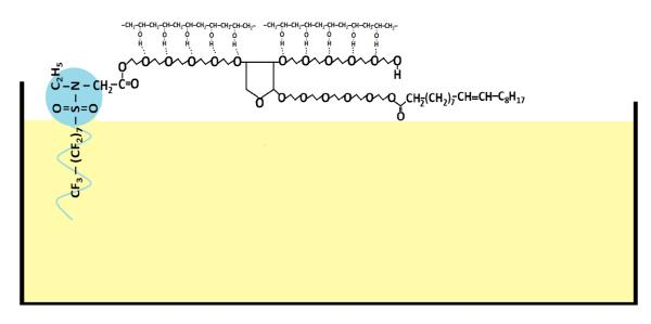
**Fig. 2**. Scheme of the coating formed by the interaction of 2- (N-ethylperfluorooctane sulfamide) acetic acid, sorbitan monooleate, polyethylene glycol and polyvinyl alcohol.
